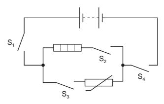
Which three switches must be closed for the heater to work?
